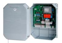
Elpro S40 electronic programmer for simultaneous management of up to four traffic control posts
